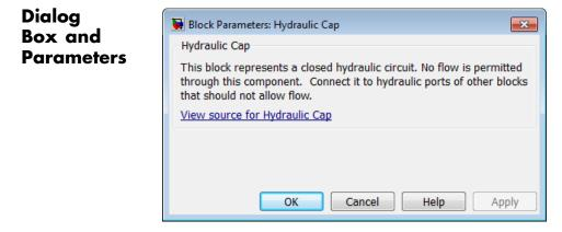
The Hydraulic Cap block has no parameters.
